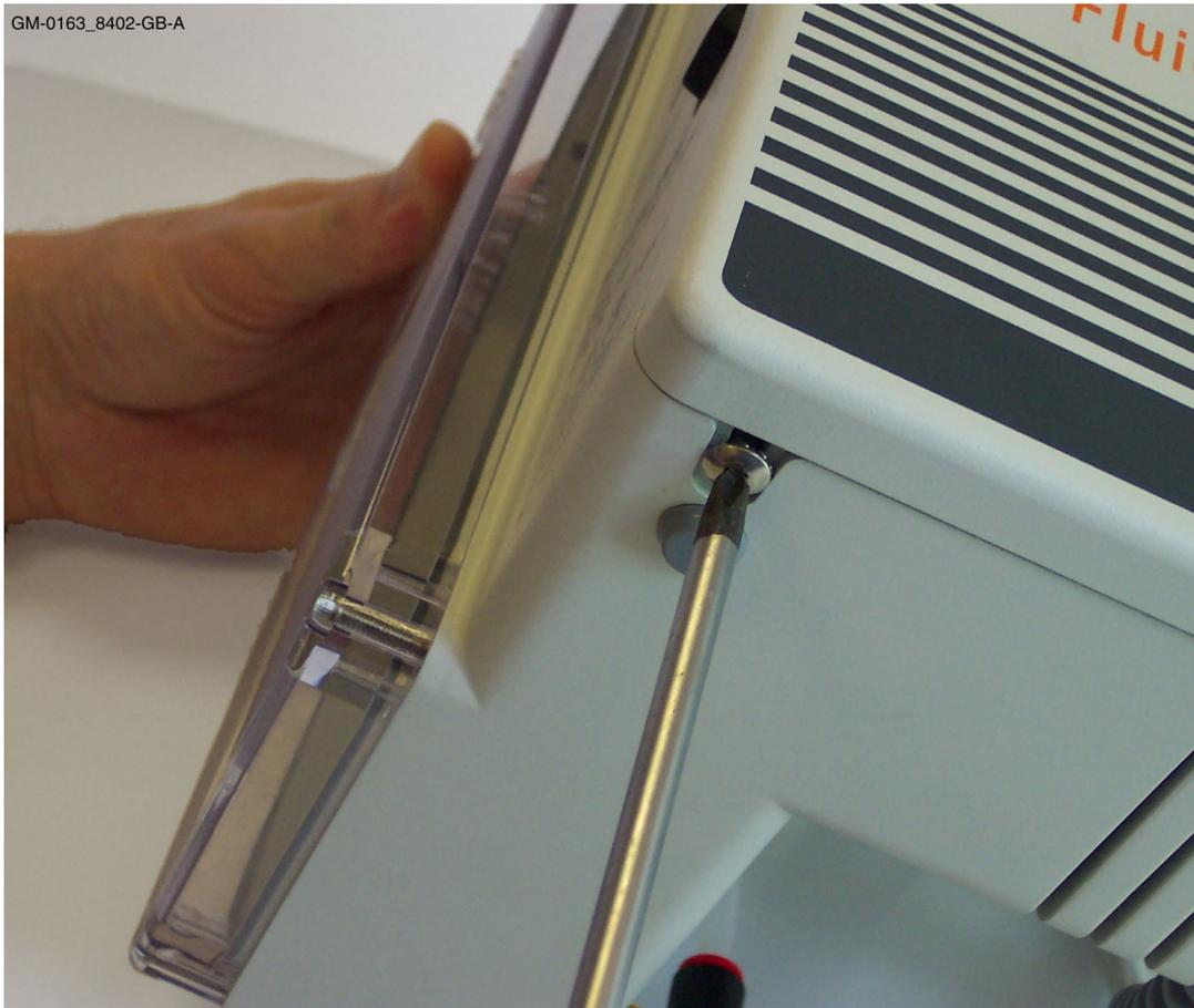
*Figure 4 - 2: Loosen, but don't completely remove these screws*
