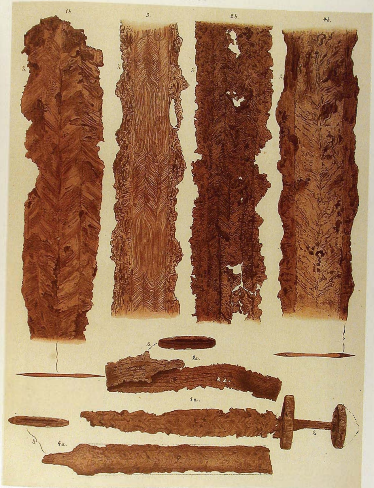
Examples of pattern-welding. Plate VI from A.L. Lorange, Den Yngre Jernalders Sværd (Bergen, 1889), reproduced at 75% of original size. The second sword from the left, Bergens Museum No. 883, has a pattern-welded core made up of three bands with aligned alternating twisted and straight areas in which adjacent bands have an opposite twist.
